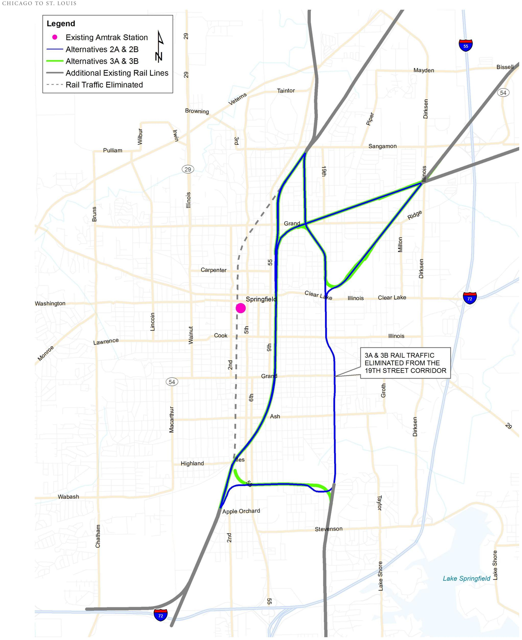
$2A \& 2B - 3^{RD}$  STREET RAIL TRAFFIC SHIFTED TO  $10^{TH}$  STREET  $3A \& 3B - 3^{RD}$  AND  $19^{TH}$  STREET RAIL TRAFFIC SHIFTED TO  $10^{TH}$  STREET ALTERNATIVES 2B & 3B HAVE ADDITIONAL GRADE SEPARATIONS
